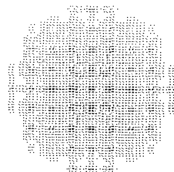
Fig. 5. Computed electron diffraction pattern for the split interstitial in gold, with relaxation.
